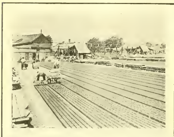
Brickyards near Haverstraw. After the bricks come from the molding and pressing machine they are placed in the sun to dry before baking.
